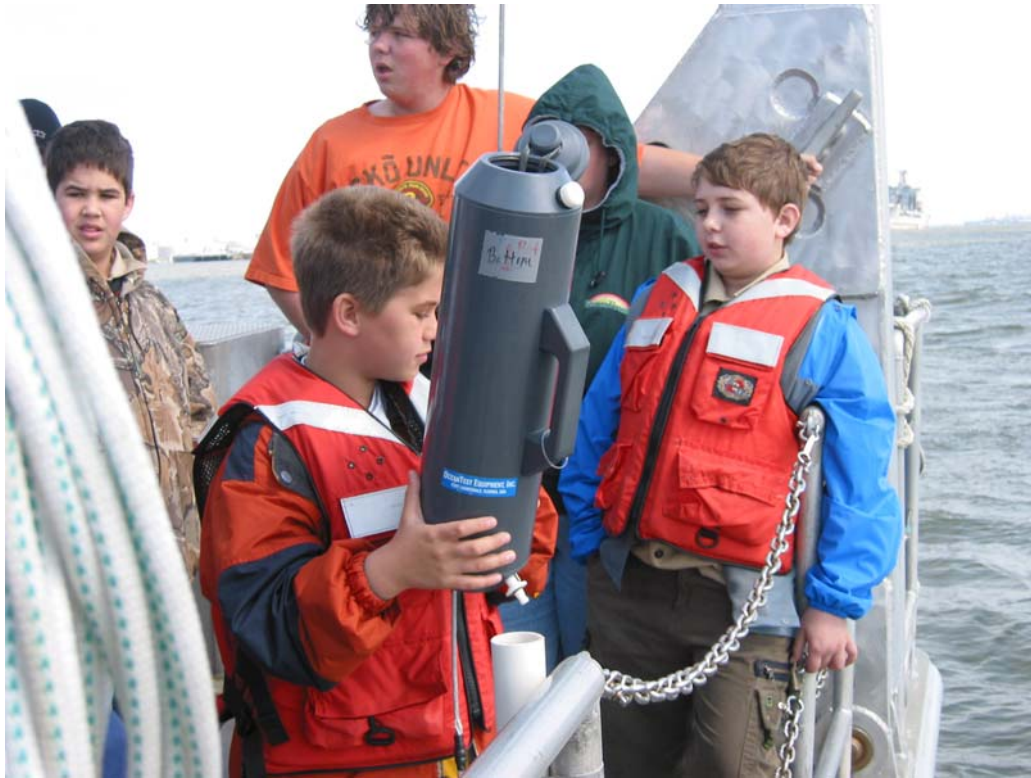
A Scout guided the Niskin bottle out to prevent it from swinging.
