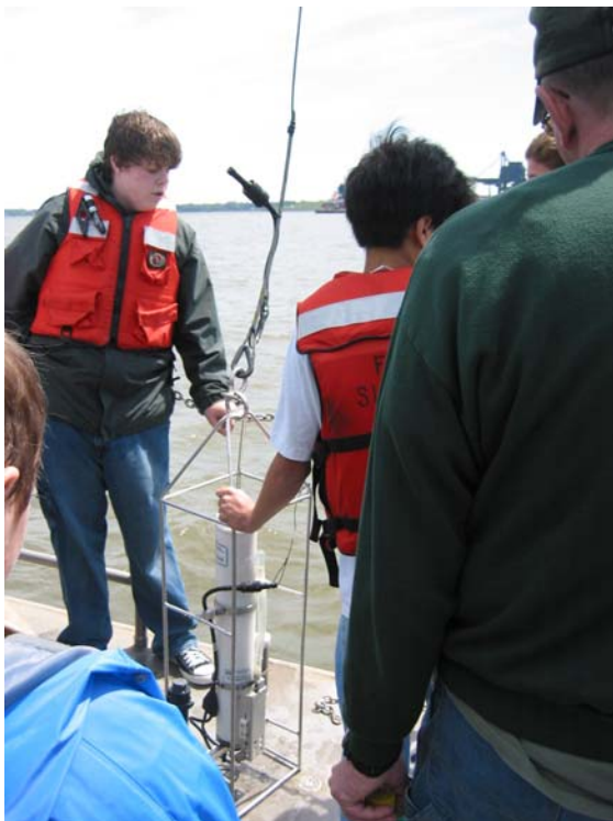
Back on deck, Scouts prepared to deploy a CTD (conductivity-temperature-depth), which measures the conductivity and temperature of the water column as a function of depth. Salinity is also measured using a CTD.
