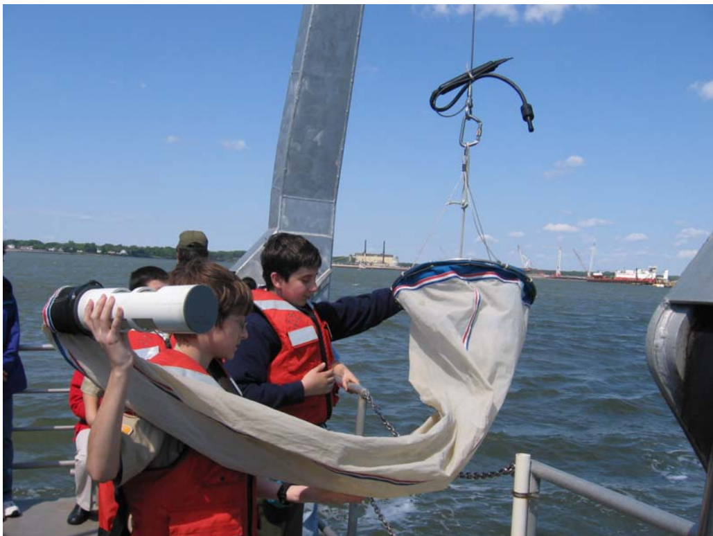
This canister, which attaches to the net, holds the various specimens collected during the tow.
