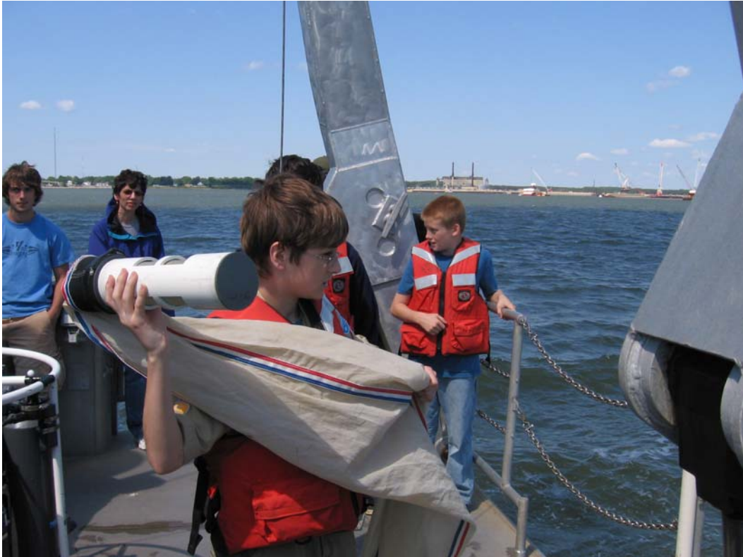
This canister, which attaches to the net, holds the various specimens collected during the tow.
