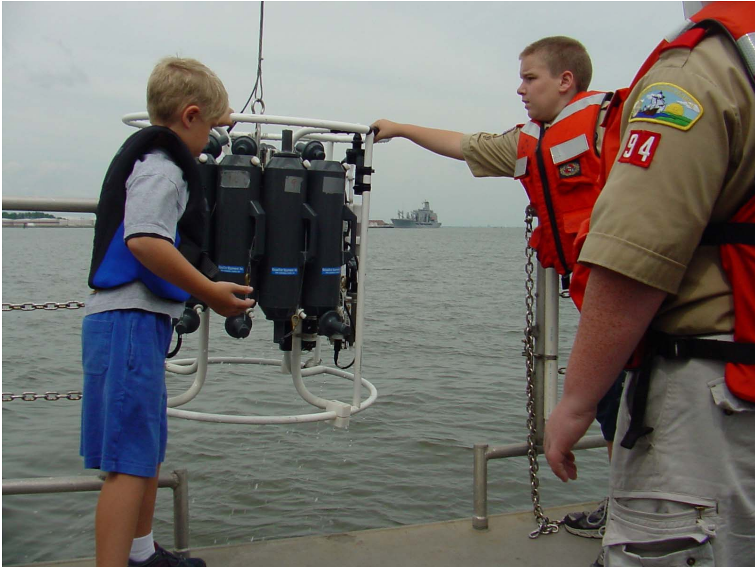
The Rosette/CTD being guided back onto the ship after the second deployment of the day.
