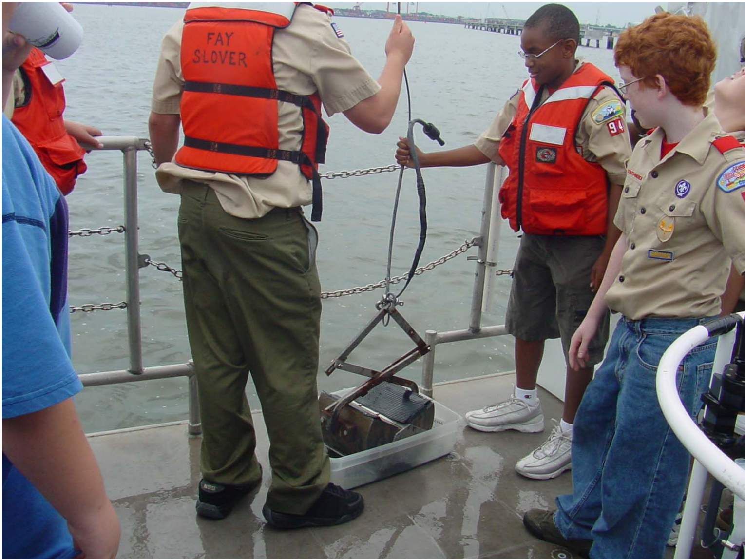
A mud grab sampler was used to retrieve sediment from the bottom of the river.
