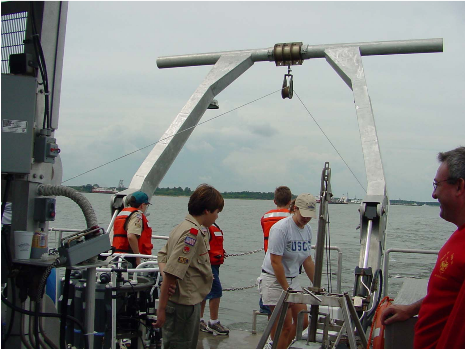
A view of the Slover's A-frame. The A-frame is raised and lowered by hydraulics, and it is used to deploy equipment.
