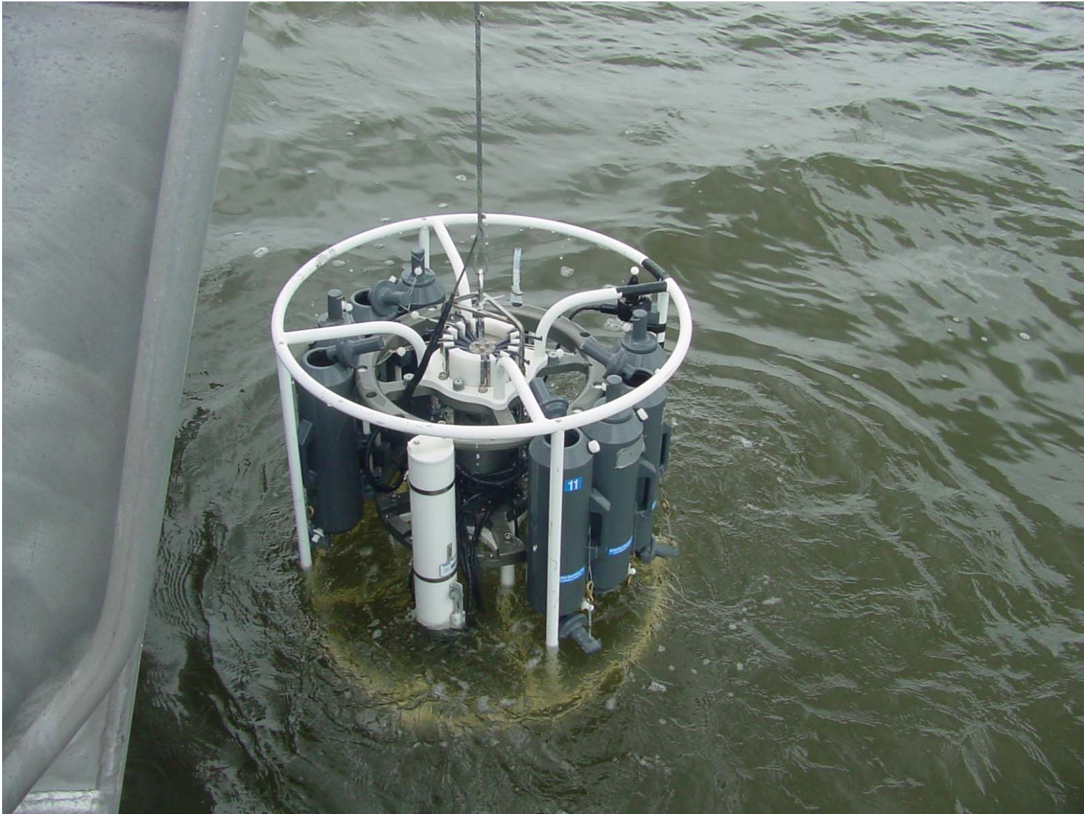
The Rosette/CTD as it is being retrieved. Notice that four Niskin bottles are closed; these contain water samples.
