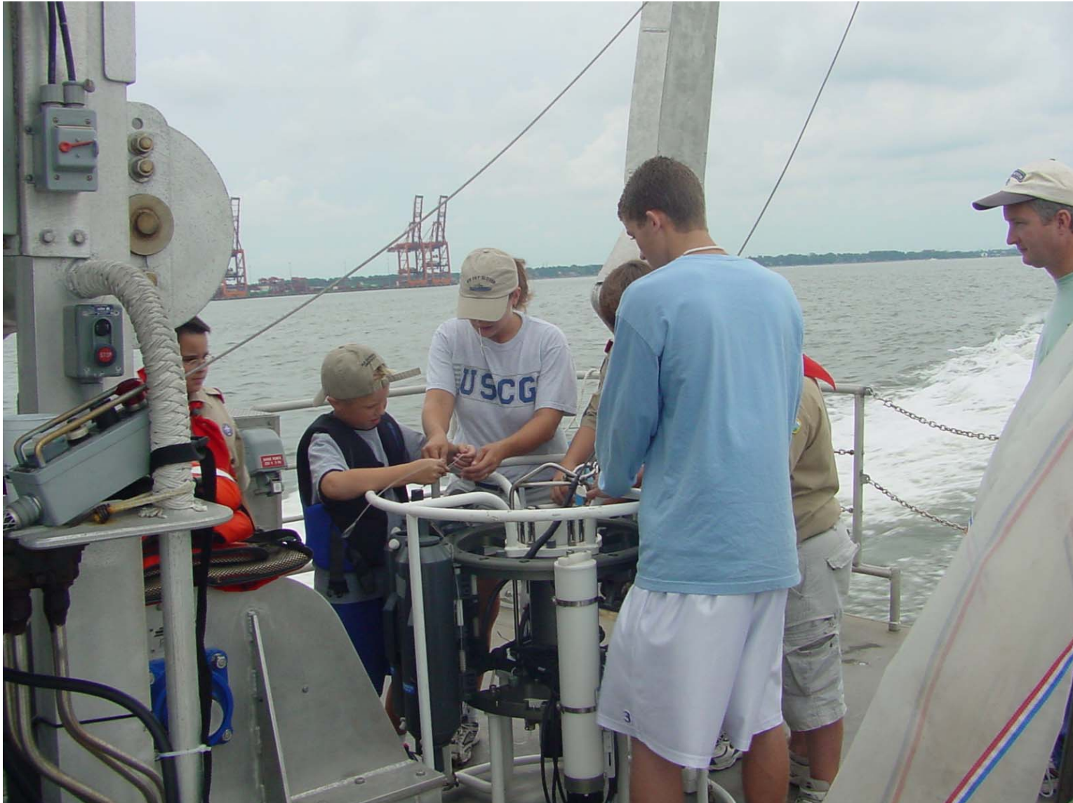
Laura instructs how to attach the “smart” cable to the Rosette/CTD before deploying.
