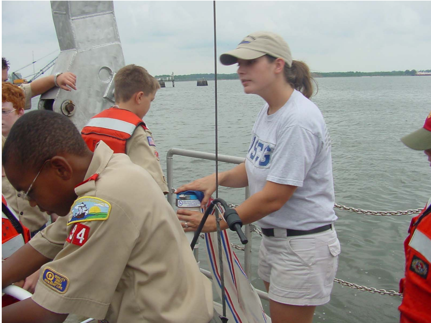
With the net rinsed, the sample jar can be detached. The rinsing helps to remove any organisms trapped in the net, allowing them to fall into the sample jar.
