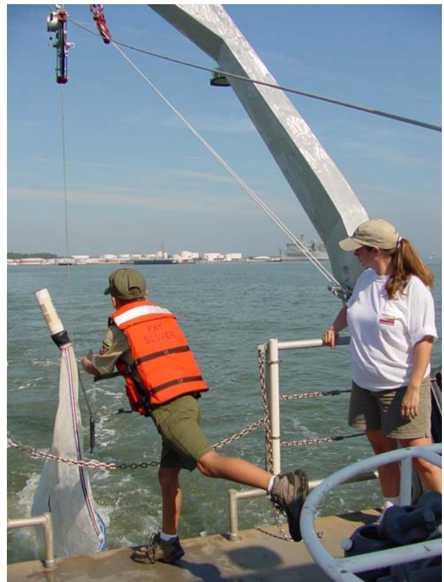
The plankton net was launched from the stern of the Slover . The attached canister collected samples caught in the net.
