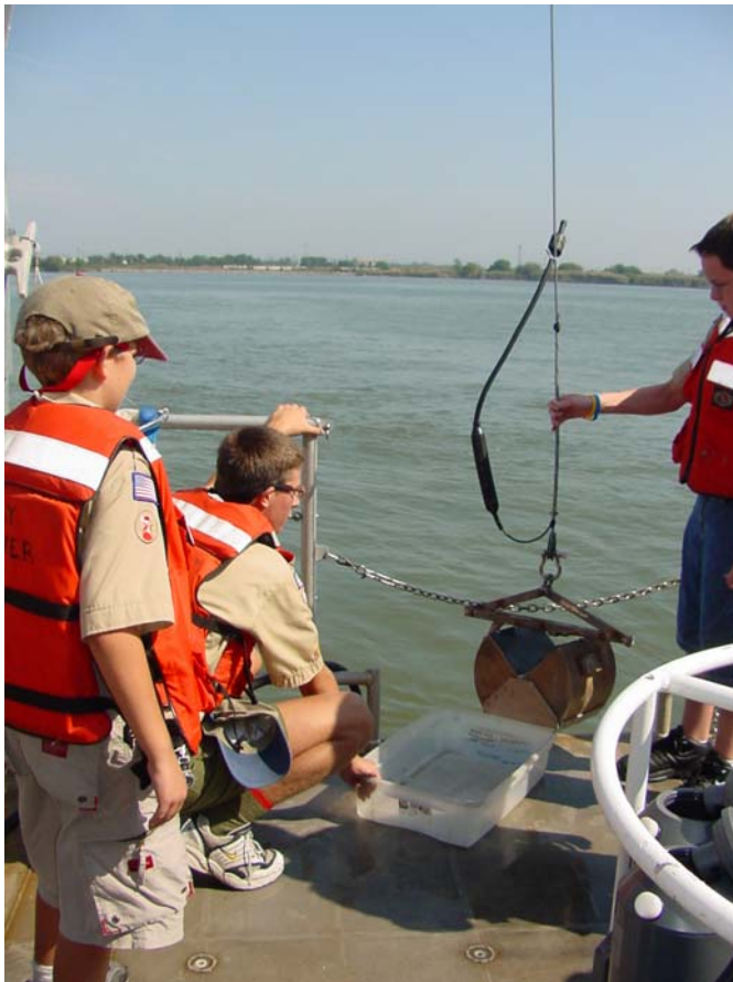
The Scout guided the cable as the equipment was lowered down to the bottom to grab a sample of mud.
