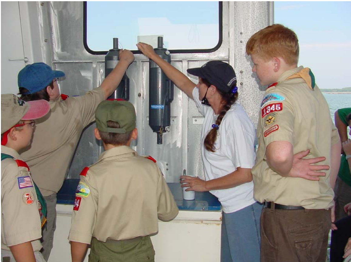
Dr. Eileen Hofmann, CCPO professor, and a Scout hung the Niskin bottles from the Rosette/CTD to drain the water for sampling.
