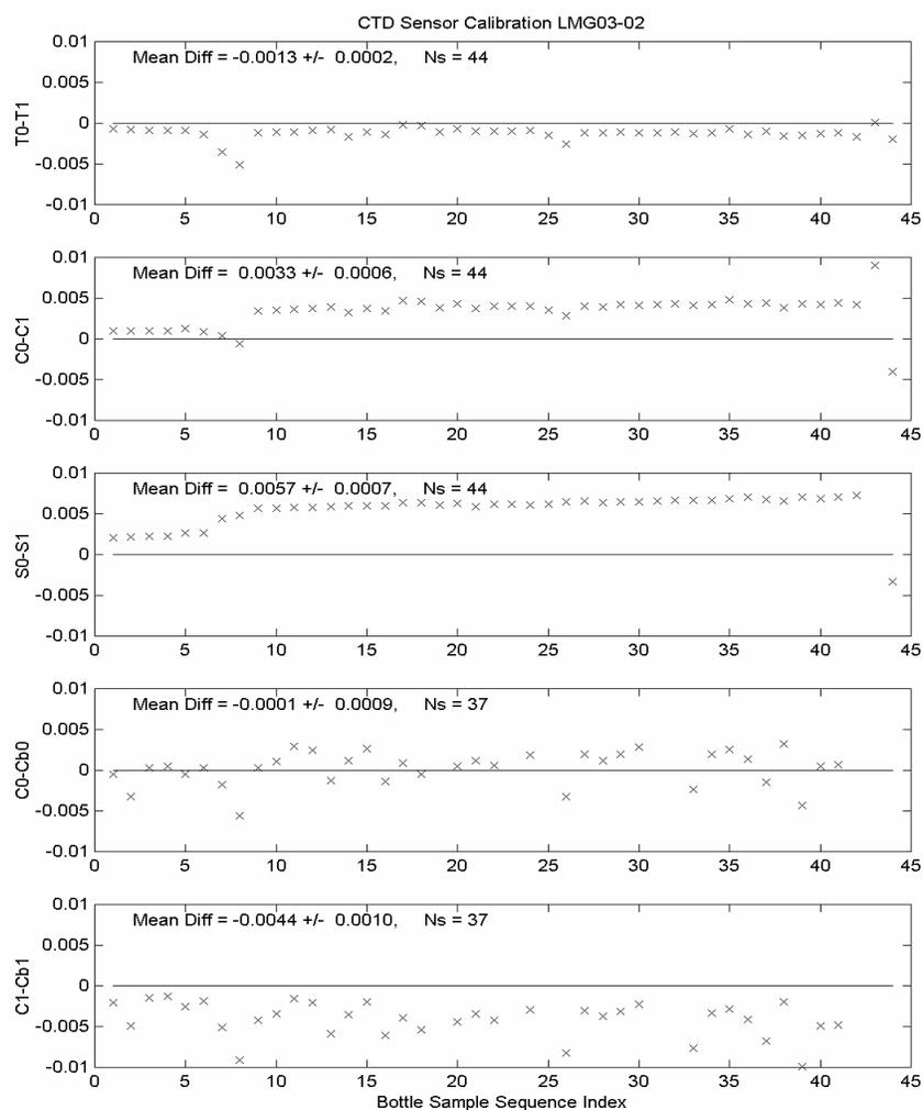
**Figure 3.** Differences between CTD primary and secondary temperatures (top panel), conductivities (second panel), derived salinities (third panel), and *in-situ* water sample conductivities and CTD primary (forth panel), and CTD secondary (bottom panel) conductivities versus bottle sample sequence number.
