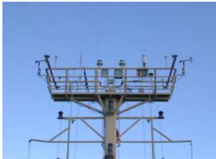
**Figure 10.** Meteorological sensors mounted on a platform railing on top of mast.
