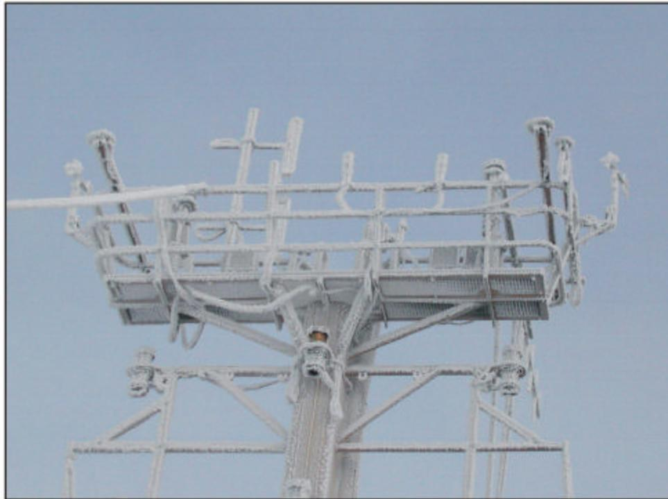
**Figure 11.** Meteorological sensors mounted on platform railing on top of the *Palmer* science mast. This photograph was taken around noon on 7 August after a night of very cold air with little wind.
