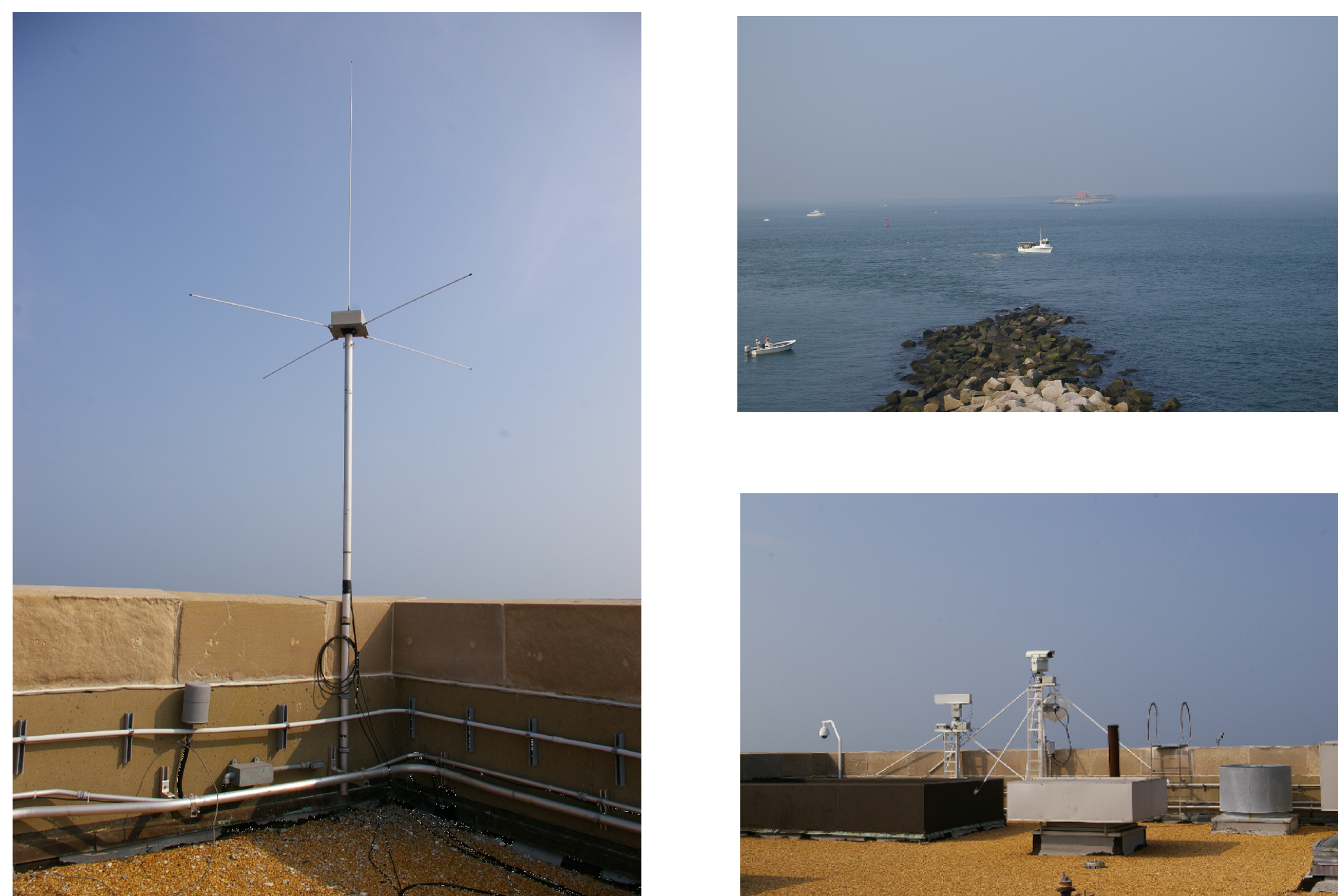
Figure 2: The CBBT antenna mounted to the roof of the fan and ventilation building at the Fourth Island (left). The south wall of the rooftop opposite the antenna (lower right) and the Chesapeake Channel (lower right).
