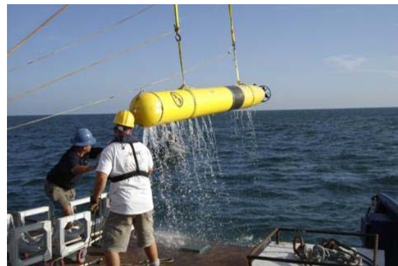
Figure II-11: An example of an underwater Automated Unmanned Vehicle (AUV). These platforms are used to survey underwater munitions safely and cost-effectively.
