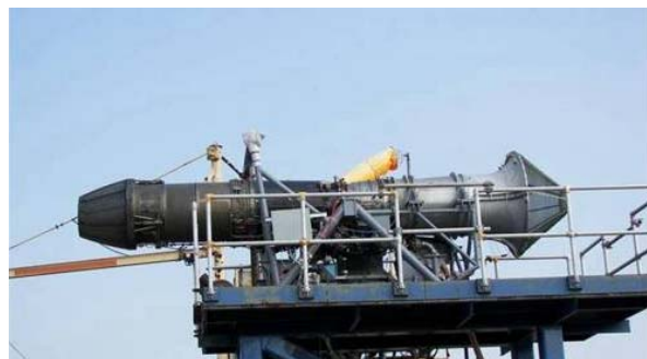
Figure II-5: Measuring the engine noise of an F404 aircraft engine on a test stand.
