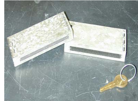
Figure II-19: Light-weight, small-form factor, soldier-portable advanced thermoelectric power system.
