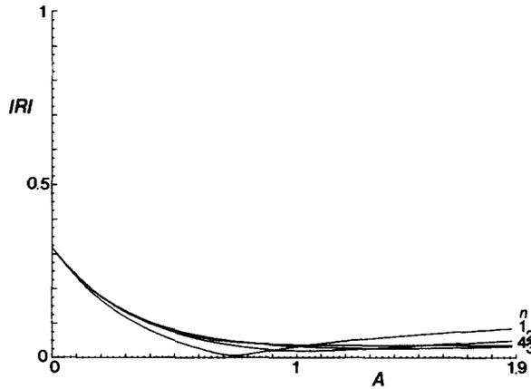
FIG. 7. Same as Fig. 6 except  $\eta = 0.5$  so a sponge filter is applied. For moderate to large  $A$ , the reflection coefficients are decreased by about a factor 2 relative to those obtained without the sponge filter.
