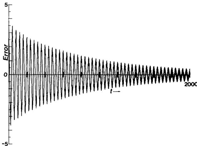
FIG. 1. A plot of the error  $v(x, t) - \sin k(t-x)$  at  $x=1$  in the solution of (3.4)–(3.6) with  $\mu = 0.1$ ,  $v = 0$ ,  $k = 2$ ,  $L = 20$  and  $0 \leq t \leq 2000$ . Here  $v(x, 0) = \frac{1}{2}x(L-x)$ ,  $v_t(x, 0) = 0$ . Observe the long decay time of the transient error to its time asymptotic value 0.18 given by (3.9). This behavior is due to the mode (3.13) with  $n = 1$ .
