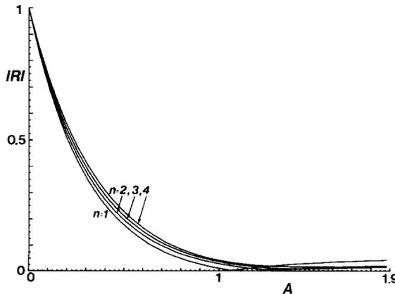
FIG. 2. A plot of the reflection coefficient  $|R|$  for the damping function (4.10) with  $n = 1, 2, 3, 4$  as a function of  $A$ . Here the reflecting boundary condition  $v(L, t) = 0$  is applied and  $k(L - x_0) = 3\pi$  so there are  $1\frac{1}{2}$  wavelengths in the damping region.
