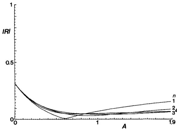
FIG. 6. A plot of the reflection  $|R|$  vs  $A$  for the model problem (6.7)–(6.8) with  $B = 0$  in (6.10),  $m = \frac{1}{2}\bar{m}, \eta = 0$  and  $v(x)$  given by (6.11) with  $n = 1, 2, 3, 4$ . Here  $m(L - x_0) = 2\pi$  so there is 1 wavelength within the damping region.
