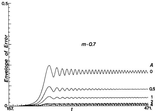
FIG. 9. Envelope of errors  $|w(x, t) - u(x, t)|$  at  $x = X - \pi$  vs  $t$ . Here  $u(x, t)$  is the solution of the Klein-Gordon equation (7.1) with radiation boundary conditions and  $w(x, t)$  is the solution of (7.3)–(7.4). Here  $m = 0.7$ ,  $k = 4$ ,  $X = 50\pi$  and  $v(x)$  is given by (6.11).
