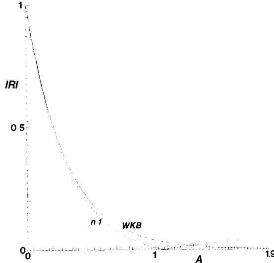
FIG. 5. Comparison between the WKB result (4.13) and the exact reflection coefficient  $R$  as a function of  $A$  in (4.10). Here the damping function (4.10) is used with  $n = 1$ ,  $k(L - x_0) = 3\pi$  so there are  $1\frac{1}{2}$  wavelengths in the damping region.
