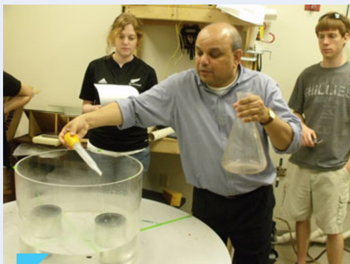
Ajoy demonstrates an experiment in fluid flows to his students, using a rotating tank.
