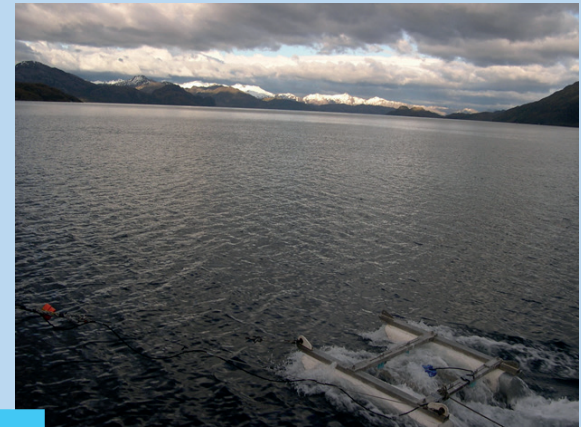
Velocity measurements being collected with a towed ADCP at a Patagonian fjord off the Strait of Magellan.
