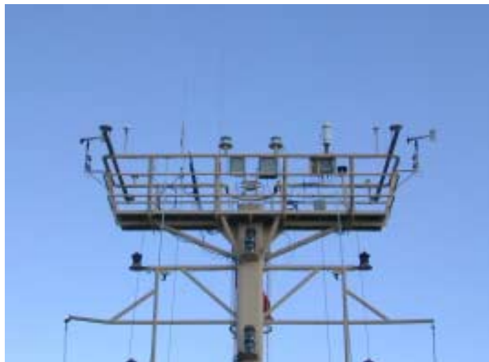
Figure 14. Meteorological sensors mounted on platform railing on top of the mast on the L.M. Gould .
