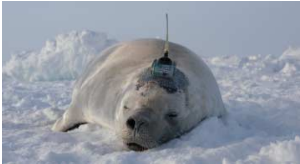
Figure 23. Crabeater seal #G42 is shown with a Sea Mammal Research Unit Satellite-linked Dive Recorder attached to its head.
