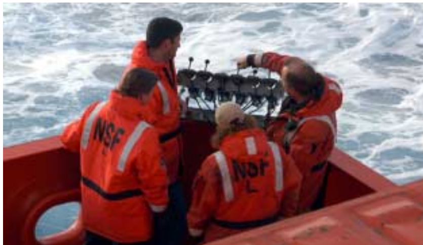
Figure 3. Andy Nunn explains how to load the launcher for XBT survey across the Drake Passage.
